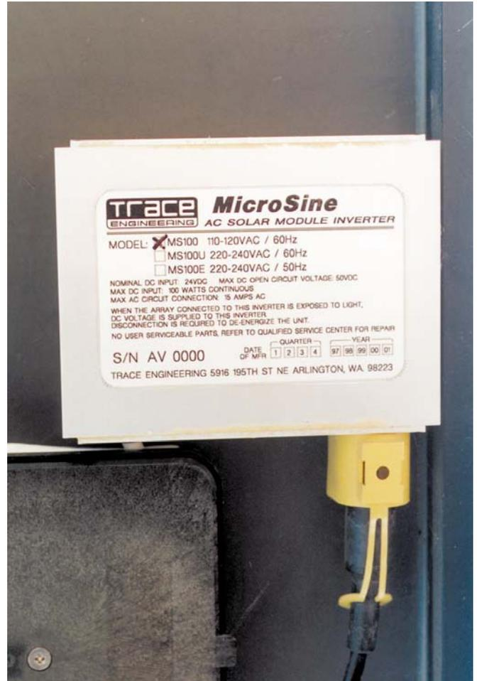
Above: The Micro Sine on the back of the 24 Volt PV.
